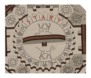
On one of the faces, below key N°2, there is a maze diagram - ?3. After completing the maze, key N°2 moves to the extreme position, unlocking key N°1. Key N°1 can be pulled upwards.
